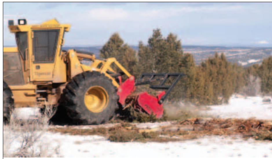
This Tigercat machine, fitted with a Fecon mulching head, grinds whole pinyon and juniper trees in a sagebrush restoration project. Photo: Tyler Thompson, Utah Watershed Restoration Initiative.
